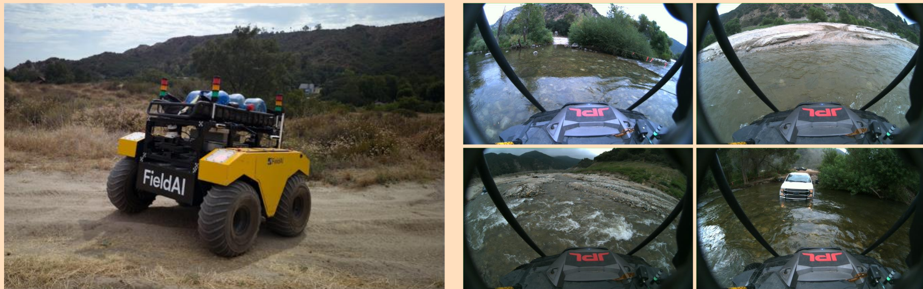
Fig 1. Examples of environmental disturbances encountered during real-world deployments. Left: A skid-steer mobile robot (SSMR) transporting a heavy payload in off-road terrain. A human operator may choose a payload with unknown mass that slides freely. In the shown case, water sloshing within the payload introduces additional disturbances. Right: An all-terrain vehicle (ATV) crossing a deep stream with strong downstream current. Although we focus on SSMRs in this work, we use this as a motivating example for the numerical studies in our work.
